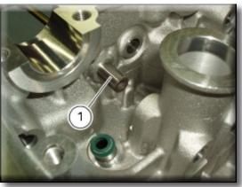
Locate the spacer (17) on the shaft.
