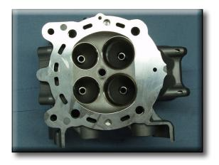
Thoroughly check the dimensions of the inner surface of the valve guide. Measure the inside diameter with a bore diameter gauge.
