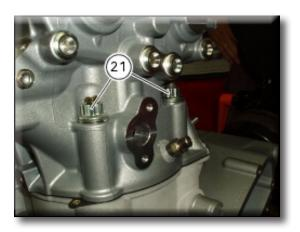
Tighten the nuts (21) on the studs in the sequence 1-3-2-4 using service tool 88713.2676 in conjunction with a torque wrench.
