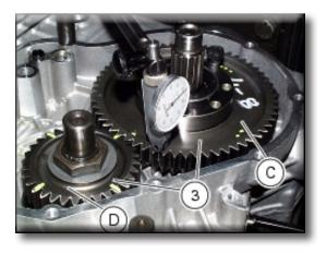
If the measured values are outside the permissible tolerance, change the position of the driven gear (C) on the input shaft leaving crankcase gear (D) untouched. If still outside tolerance values, renew the primary drive gear pair.
