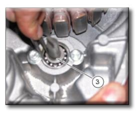
Recover the ceramic washer (A) and seal ring (B) located on the inner side.
