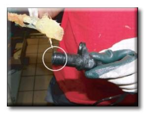
Fit the engine sensor (23) in its seat in the crankcase.
