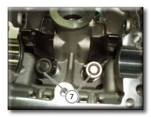
Install the closing shims on the intake valves (14) using the method described above for the exhaust valves. Refit the camshafts to check the valve closing clearances.
