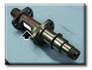
Lubricate with the specified lubricant (Molycote M55 Plus), the camshaft seats on both the cylinder head and the supports (22) and (23) (green zone).
