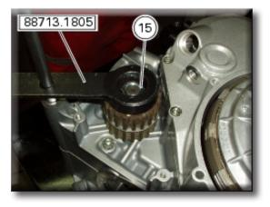
Remove the nut (15), the spacer (20) and the outer pulley (18).
