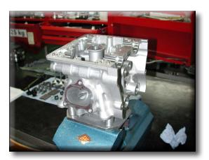
The intake side can be identified by the presence of four threaded holes on the flange.
