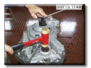
Remove the gearbox shafts and gear selector drum from the crankcase halves.
