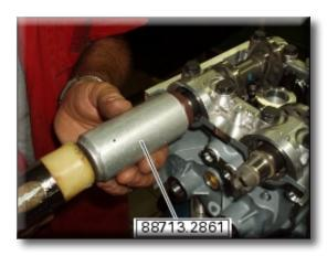
When correctly installed, the oil seal should be flush with the bevel of the cylinder head bore.
