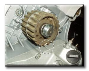
Install the service tool 88713.2011 in the alternator cover to hold the crankshaft against rotation and secure it the relative pin.
