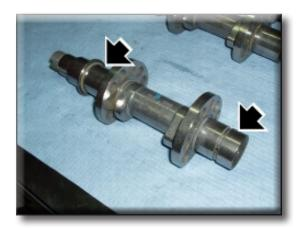
Visually inspect the camshaft tracks for scoring and abnormal wear. If any of the above defects are found, the camshaft should be renewed.
