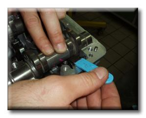
In this condition, with the piston of the horizontal cylinder at TDC with the valves fully closed as confirmed by the reading on gauge (G), set the gauges (H) to zero.
