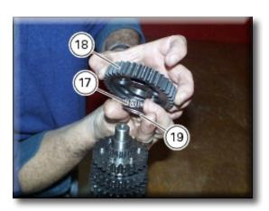
Remove the fifth speed driven gear (20).
