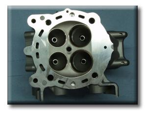
Minor damage can be repaired by grinding with special  $45^{\circ}$  and  $60^{\circ}$  single-blade grinders. Grind the valves and check the seal.
