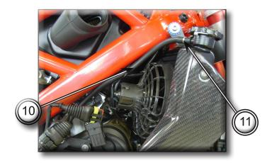
Unscrew the three screws (25) then remove the expansion tank (1) together with the plate (3) and the hoses (10).
