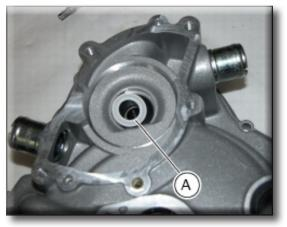
Insert the impeller shaft (10) with the mechanical seal (9). Turn the cover over.
