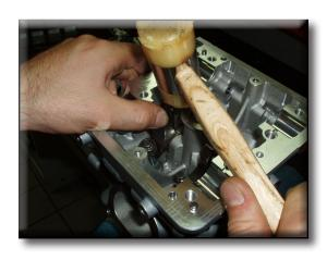
Repeat the procedure with the opposite valve and check that the top of the valve stem is aligned with the surface of the shim (7); if it is not, repeat the half-ring installation procedure.
