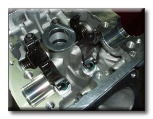
Using an M5 bolt, withdraw the shafts (1) of the closing rocker arms on the exhaust and intake sides.
