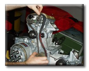
Fit the tensioner pulleys (9) on the mounting studs on the two cylinder heads. Start the nut (8) on the crankshaft
