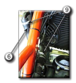
Loosen the clamps (9) and the clamp (15), disconnect the wiring connector (4) of the temperature sensor from the electric wiring then remove the vertical cylinder hose (8).
