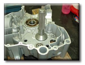
On worn engines, the bearing holder may no longer be a tight fit in the crankcase half.
