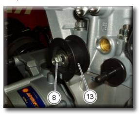
Unscrew the bolts (22) securing the pulleys, turning them anti-clockwise through  $90^{\circ} \pm 5^{\circ}$ . Check that the pulleys have no endfloat and can rotate freely at all points along the full length of the slots.
