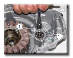
Now turn over the cover and fit the locating ring (8) using drift part no. 88713.0870. Position the ring as shown in figure and push it until it seats against the spacer (7).
