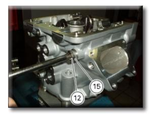
Using an M5 bolt, withdraw the shafts (2) of the opening rocker arms (3) on the exhaust and intake sides. Remove the opening rocker arms (3).
