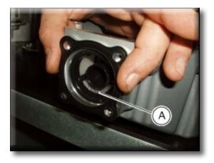
Remove the drain plug (10) with its seal (9).
