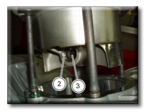
Working from the opposite side, drive out the gudgeon pin sufficiently to release the connecting rod. Lift the barrel/piston assembly clear of the crankcase studs. If work is to be carried out on the piston, carefully withdraw it from the cylinder.
