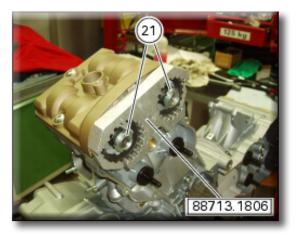
Using the bush supplied with service tool 88713.1806 and a torque wrench, tighten the nuts (21) to their specified torque.
