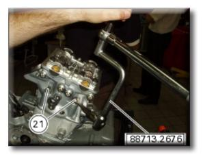
Remove the cylinder head nuts (21) and special washers (22).
