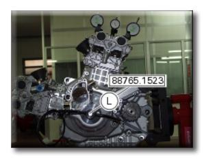
Remove all tools installed for the timing check and tension the belts to their prescribed operating tension, as described in "Measuring timing belt tension".
