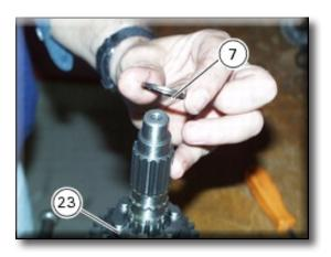
Remove the circlip (7) and withdraw the splined washer (6) and the second speed driven gear (24).
