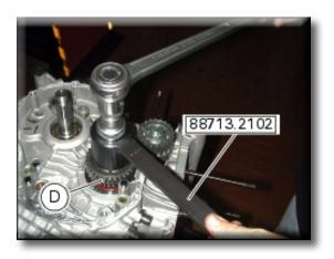
Stake the washer (10) on the gear (D) in correspondence with the milled location and on the nut (11) in a diagonally opposed position.
