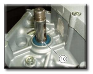
Install the inner spacer (17) on the driveshaft, taking care to align the notch in the spacer with the slot for the Woodruff key.
