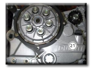
Unscrew the retaining bolts (4) and remove the collars (2) and the clutch springs (1).
