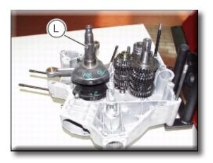
Remove the timing belt driveshaft (30).
