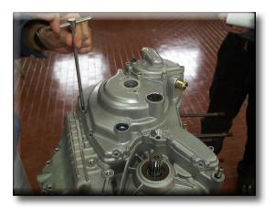
Re-use the left-hand crankcase cover or a service cover with puller 88713.1749. Secure it to the crankcase half using some of the original bolts and begin separating the crankcase halves by turning the central pin of the tool. Tap the end of the gearbox output shaft with a plastic mallet to separate the crankcase halves.
