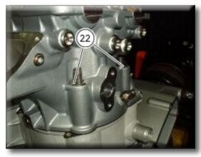
Remove the cylinder head assembly by lifting it off the engine studs. Repeat the same procedure for the other cylinder head.
