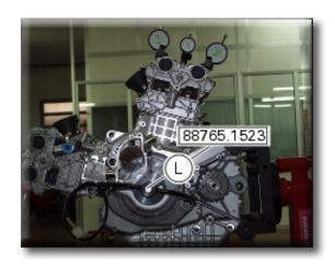
Set the opening valve clearance to zero when the camshaft is in its rest position by fitting a feeler gauge between the upper rocker arm and the opening shim.
