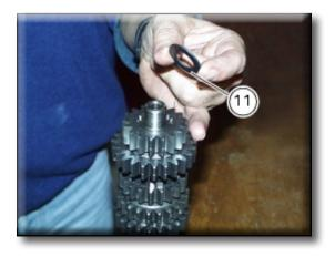
Remove the second speed driving gear (10). Use two screwdrivers to prise out the circlip (7) and the splined washer (6).
