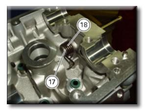
Locate the closing rocker arm (16) and drive the shaft home.
