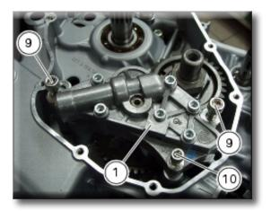
Check the gear backlash with the driving pinion by fixing dial gauge part no. 88765.1518, equipped with the relevant stylus, to the crankcase.
