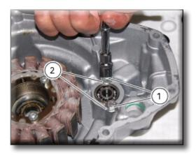
Working from the rotor side use a suitable drift to press on the inner race of end bearing (5) until it can be extracted from the cover. Use the same technique to remove the other bearing (6).
