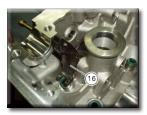
Proceed in a similar manner to install the closing rocker arm (4) with the spring (19) from the exhaust side.
