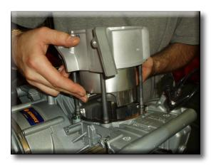
Remove the four O-rings (A) located on the crankcase studs between the barrel and the base gasket (5).
