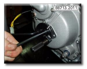
Fit the service tool no. 88765.1524 to prevent rotation of the camshafts: one for the vertical cylinder head and one for the horizontal cylinder head.
