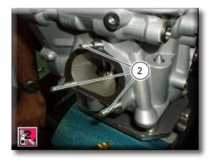
Check that the camshafts (marked "VA" and "VS" for the vertical head and "OS" and "OA" for the horizontal head) are clean and in good condition. If the camshafts are not new, use emery cloth to remove signs of wear on the cam and support surfaces, working on a flat surface.
